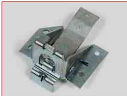
The lock lever, the part of the latch that has the hole with a new edge can be bought separately for about \$35 each, but now you have a shiny lever inside old latch housing. There's also a left and right.
