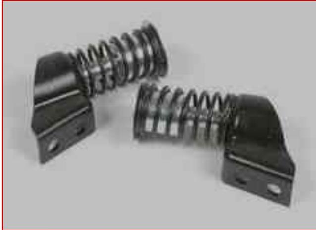
Trial cutting of the repro springs is needed to get the right fit, but cut too much and it won't do its job as needed, leaving the front edge in danger against the hood surround when the hood is raised. 🚗
