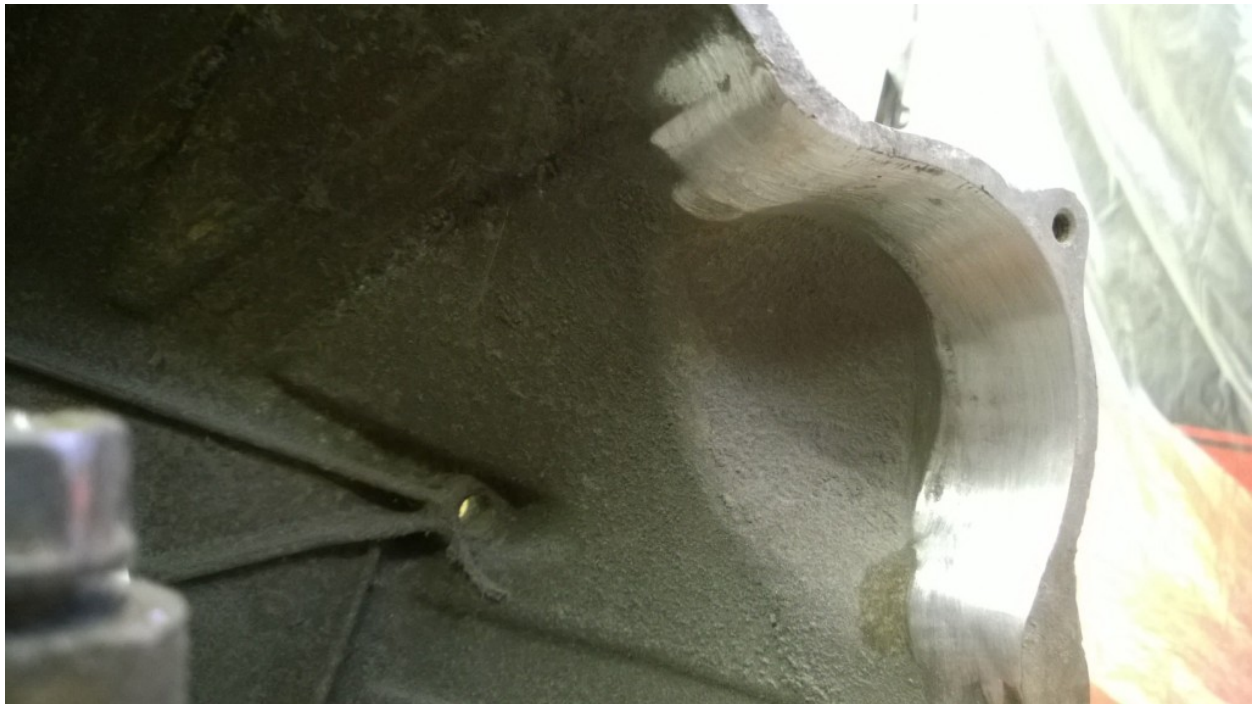
You need to use a die grinder to add clearance for a stock type starter nose. If using a mini starter this is not required.
