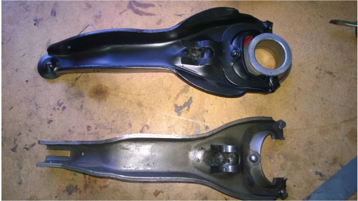
1983 Camaro clutch fork on top (Pioneer P/N CF100), stock '67 Corvette fork bottom.
