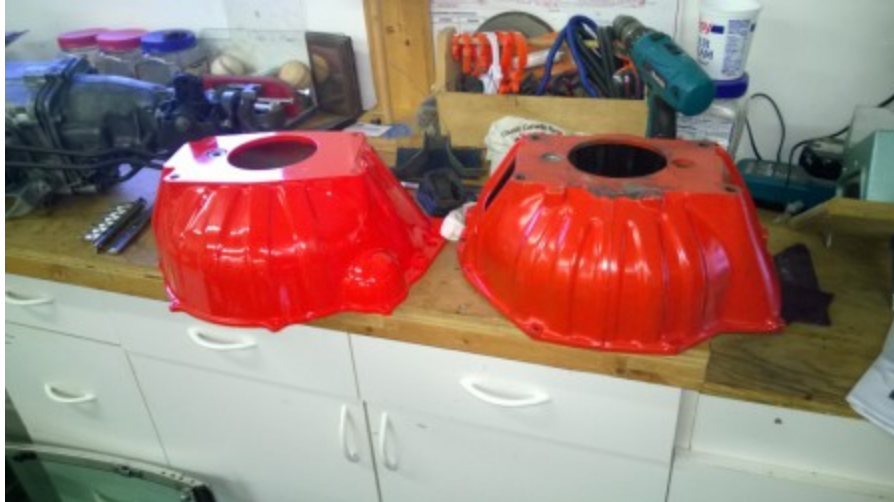
1983 Camaro bellhousing with 18 degree tilt on left compared to the stock Muncie bellhousing.
