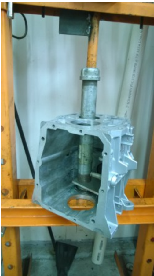
Start by pressing in new front bearing race.
