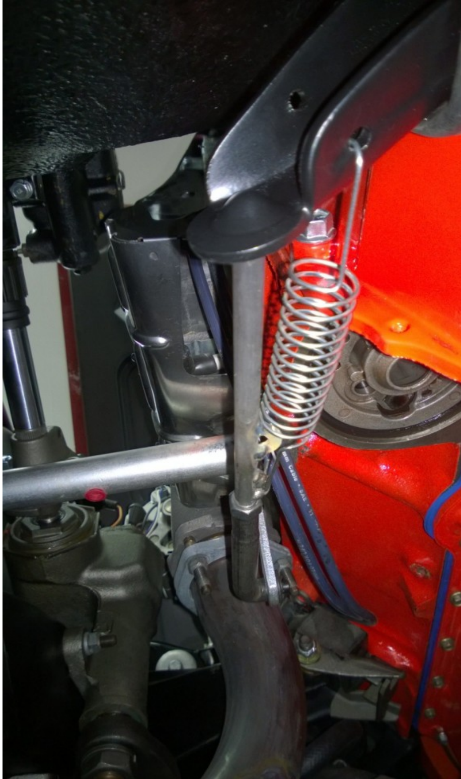
Modified pushrod installed. By using the '83 Camaro clutch fork you have a perpendicular attachment at both the Z bar and clutch fork. The clutch pedal feel is just like before with the Muncie linkage.
