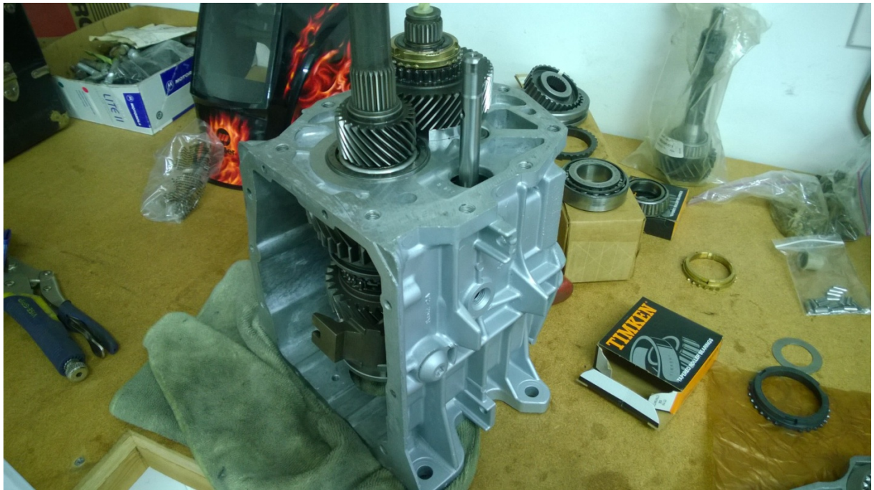
Assembly of the main case with counter gear shaft, main shaft and 5 th gear installed.
