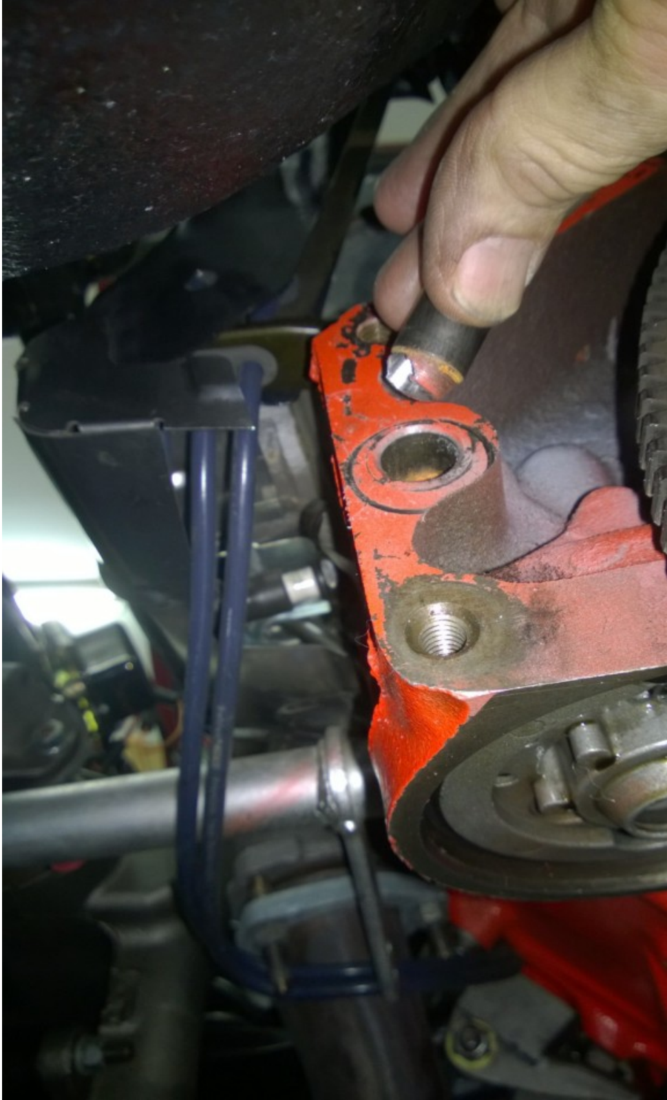
Removing factory dowel pins. This required drilling and tapping in order to pull them out.
